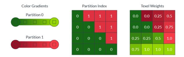
ASTC allows a single block to reference up to four color gradients, called partitions. Each texel is then assigned to a single partition for the purposes of decompression.
